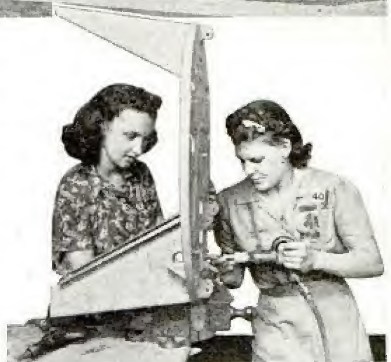
Girl at left bucks rivets driven by gun at right in assembling fuselage bulkhead for a Vultee plane
